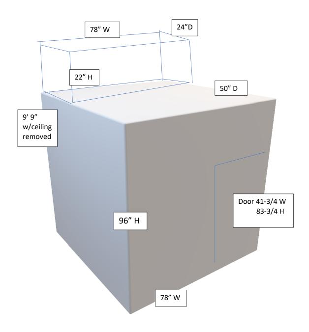
The ceiling in the elevator can be removed, which opens up an additional area. It allows items up to 9'9" to be loaded,
